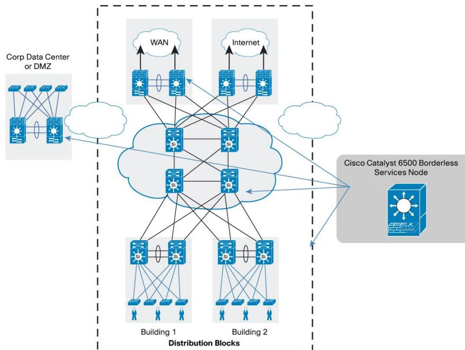
The integrated switching and services design enables you to install this node easily in your current deployment, it saves rack space, and it helps to reduce total cost of ownership (TCO). The VSS enables load sharing and increases network availability.
